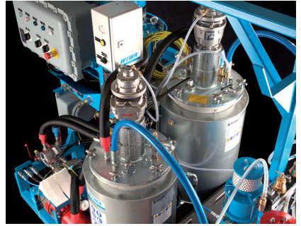
DUOMIX 333 PFP -Zone 1- pneumatic agitators
